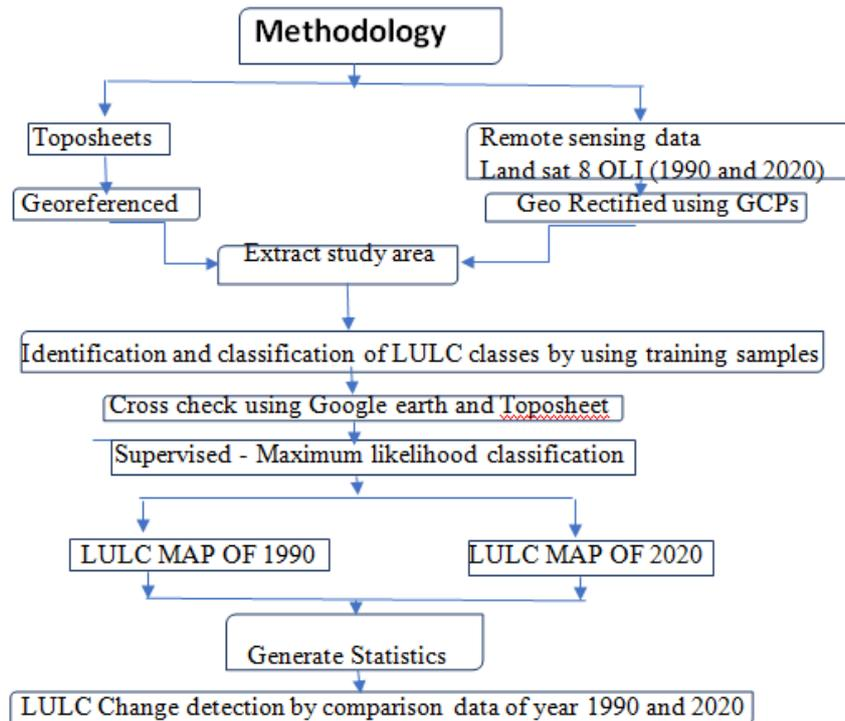
Figure 2: flow chat of methodology for LULC change detection
